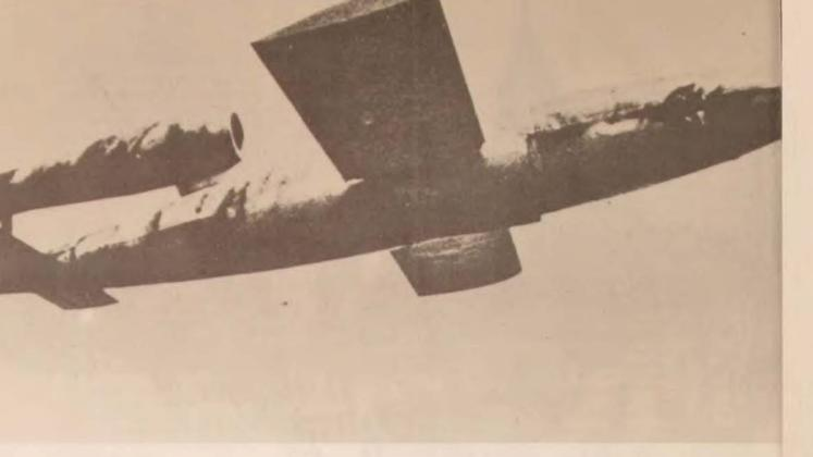
The German V-1 was a cheaply built and cost-effective "flying bomb." The pulse-jet power plant was inexpensive, yet gave the missile a top speed close to that of pistonpowered fighters. (Imperial War Museum).
