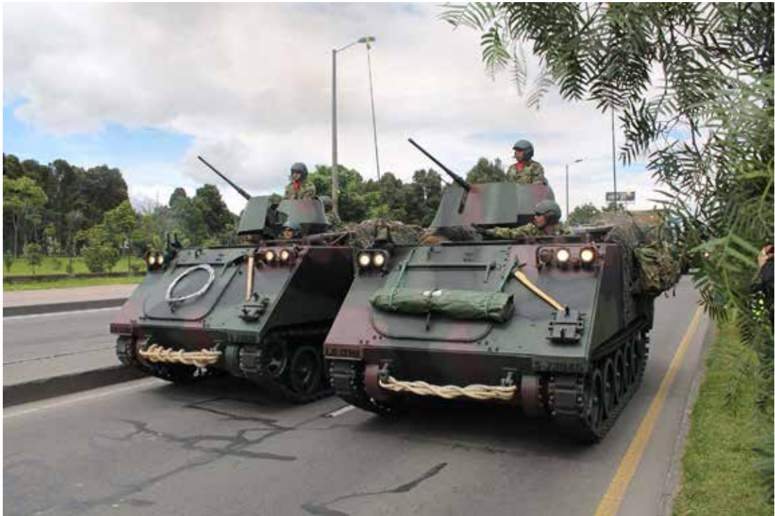
M-113A2+ of the Colombian Army. From the image you can see they are in perfect condition. These vehicles are with the Mechanized Infantry in the northern part of the country. The modernizations made them lose their amphibious capability. The only armored amphibious vehicles that the Colombian Army now owns are the EE-11 Urutú.
