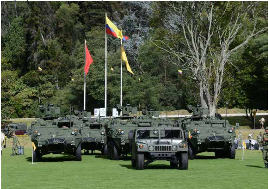
Mechanized Infantry Unit of the Colombian Army made up of five 8x8 LAV-III y one HMMWV. The LAV-III is equipped with an automatic turret, Rafael, of Israeli manufacture, "Remote Controlled Weapon Station" (RCWS) Samson Mini, with a .50 caliber (12,7 mm) weapon.
