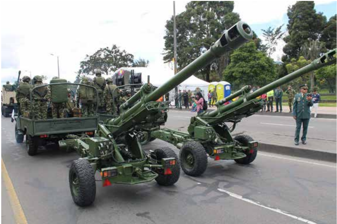
LG-1 105 mm. howitzer, being towed by M-462 Abir vehicles. The Artillery Batteries with these weapons have modern systems of firing control, data links and target acquisition. However, they are considered extremely light and the crew is unprotected when facing counter fire, therefore Colombia needs self-propelled artillery weapons.
