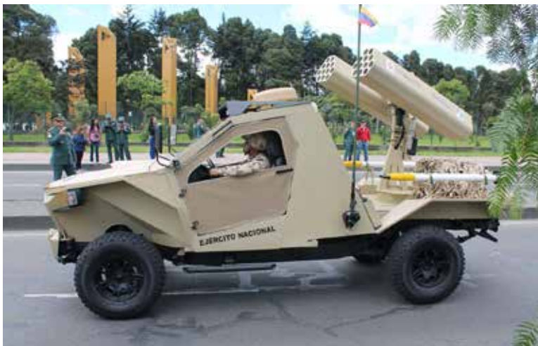
Cobra is a vehicle designed and manufactured nationally, this a multiple rocket launcher 70 mm. version. This version has been widely tested and has given excellent results. We hope the Colombian Army purchases them to equip artillery units.
