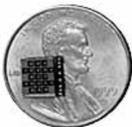
Figure 3.1. Northrop Grumman prototype of a digital microthruster array. (David Lewis, “MEMS/Micropropulsion,” Northrop Grumman Corp., http://www.st.northropgrumman.com/capabilities/space propulsion/technologies/micropropulsion.html .)
